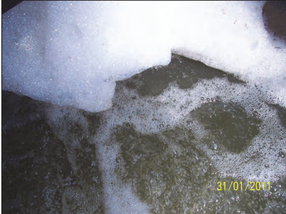
Photo 1: Pollution Incident in Toray Bioreactor. 31 st January 2011
