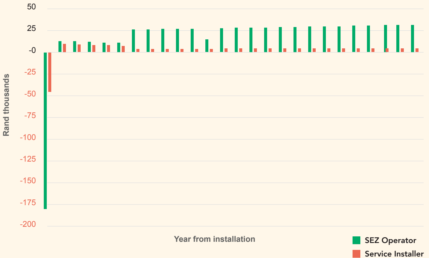
Figure 4: Annual cumulative payback model of the solar PV system from energy sales at a breakeven point of 10 years
